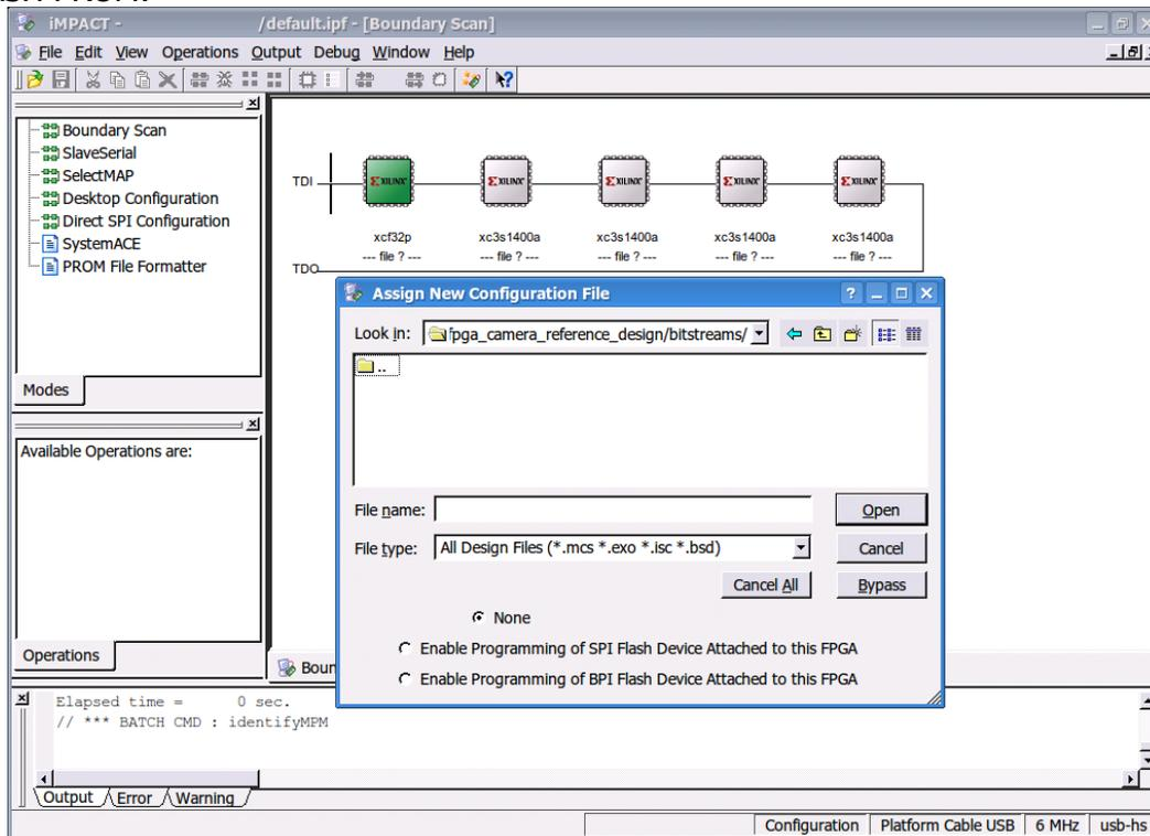
The currently selected device is shown in green. The default configuration files are available in the folders vdfpga\_camera\_reference\_design/ and vdfpga\_camera\_reference\_design/bitstreams/
